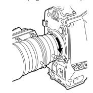
4 Press the cable into the cable clamp and connect it to the LENS connector.
